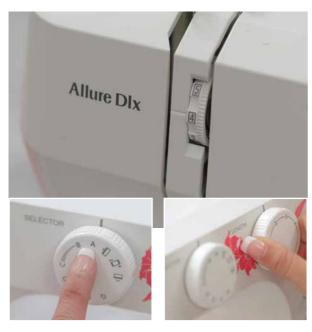
Set your machine -- turn the Thread Tension dial to 4, select A on your Pattern Selector Dial for Straight Stitches, and set the Stitch Length at two and a half.
