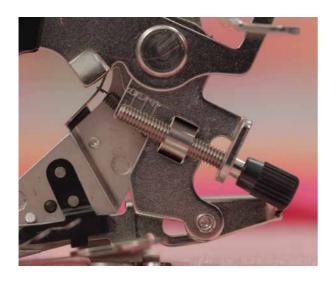
This black screw here is the Ruffling Depth Screw and it allows you to adjust the depth of the pleats. 1 is for really tiny pleats. 4, 6, and 8 increasingly make deeper pleats.
