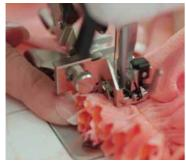
Feed the 1st strip of fabric into the Ruffler Foot's slit like this, and begin sewing.
