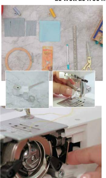
The darning foot ensures proper stitch formation and minimizes skipped stitches while protecting your fingers as you move the fabric freely under the needle.
