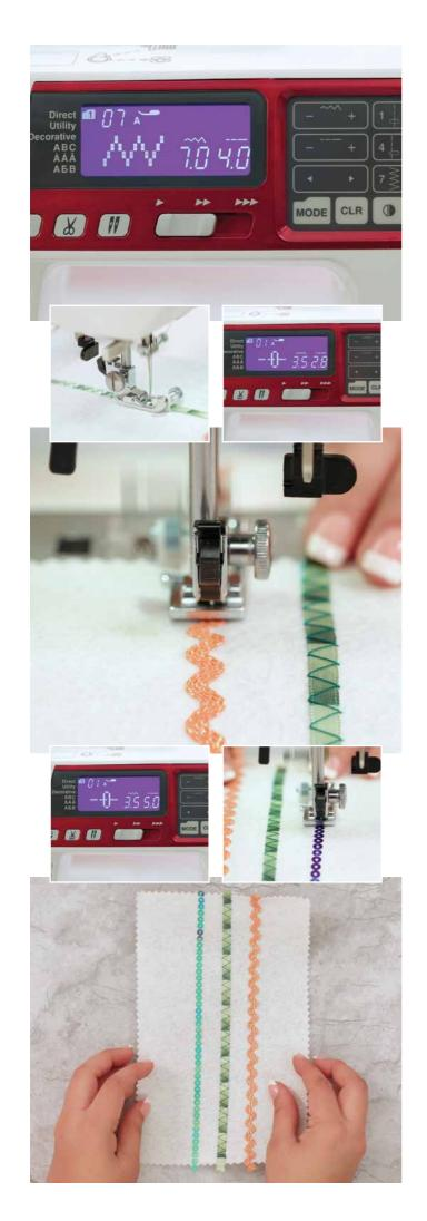
Let's start with the ribbon -- insert the ribbon into the slot in front of the foot and lower the presser foot.
