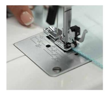
Pass the extra thread gently under the pressure foot and carefully curl the stitched fabric and pull it with the thread tail. Slowly run the machine so that fabric enters the Picot foot and starts curling.
