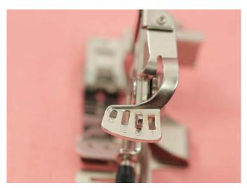
This here, is the Ratchet Gear Feed plate.
