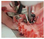
Feed the 1st strip of fabric into the Ruffler Foot's slit and begin sewing. Next, let's try out the 6 stitches slot, by moving the Ratchet Gear Feed plate. Feed the next strip of fabric you have into the Ruffler Foot's slit and sew to get a ruffle after every 6 stitches. Now move to the slot numbered 12. Feed the third piece of fabric and begin to sew.
