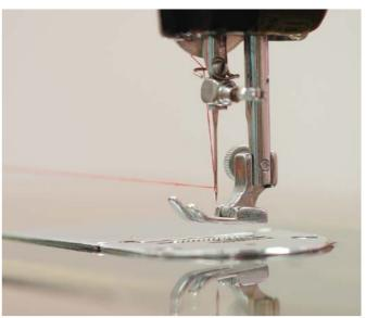
And start the machine – when the bobbin is fully wound, it will stop automatically. Cut the thread. Remove the filled bobbin and tighten the stop motion. Now here – Place the bobbin into the bobbin case like this, now here make sure the thread unwinds in the clockwise direction. Pull the thread into the bobbin case slot. Then draw the thread under the tension spring and into the delivery eye while leaving about 10 cm that is (4 inch) of free thread.
