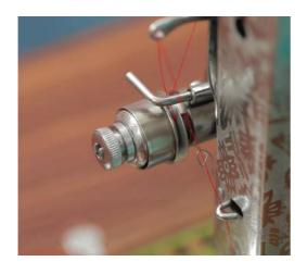
This is how you adjust the Thread tension for the upper thread. Move the Thread tension knob like this for loose tension and like this for tight thread tension... This plays a very important part in defining the final finish of the stitches. The thread tension needs to be just right...if it's loose you will find extra thread bunched up in every stitch making it very unsightly, and if it's too tight then the thread will keep breaking.
