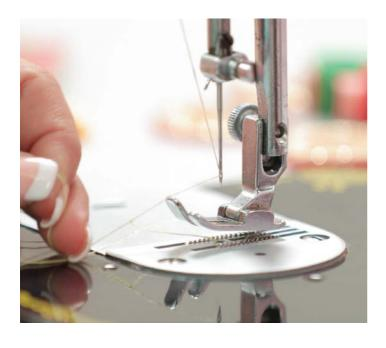
This is the Needle Plate, which brings the threads from the needle and bobbin to form the stitches.
