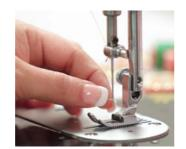
And next pass the thread through face plate thread guide like this. Next draw the thread down and slip it into the needle bar thread guide. Now for that final step -- Insert thread into the needle eye from left to right. Hold the needle thread in your hand move the flywheel towards you till the Needle goes down fully and comes out of the needle plate. Pull the thread in your hand to draw the bobbin thread out.
