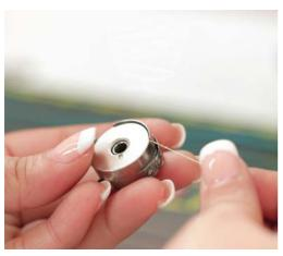
Now that you know how to remove the Bobbin Case. Take it out and slide out the bobbin from it. Now place the thread spool on the spool pin as I am doing with the thread coming from the back of the spool
