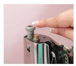
This brings us to the Pressure Bar Thumb Screw; it enables adjusting the pressure exerted by the presser foot on the fabric.
