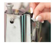
Draw thread through the check spring at this point. Then take the thread through the thread take up lever as you can see me doing.
