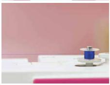
To do this you first need to remove the bobbin from the bobbin holder. Select the Lockout key to lock the machine. Slide the hook cover release the button to your right to release the hook cover plate and remove the bobbin.
