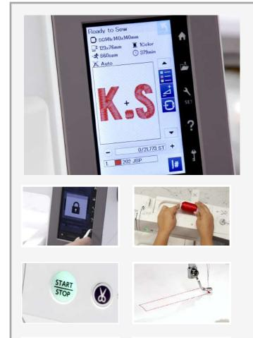
Lets look at the details of this design. The hoop size as mentioned earlier is Sq14b which is 140 x 140 mm. The size of the embroidery is 123 x 76mm. The speed of the machine or the stitches per minute are 860. Our monogram is using only one red color. The entire design is going to take 379 mins. This at the bottom is the stitch count. The entire design will take 21,773 stitches. The last row shows the colors which is recommended by the machine according to our design.
